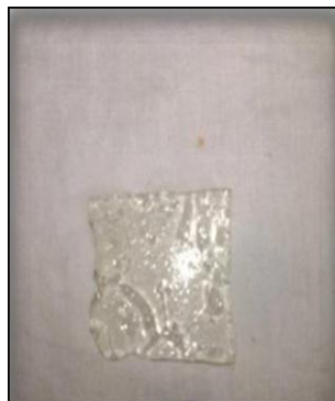
Figure 7 (b). Integrity of PG-3 film at pH 9.2.
