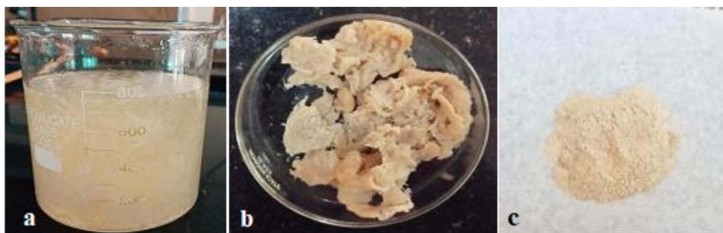
Figure 1. Mucilage obtained after hot extraction (a), precipitated by ethanol (b), dry powder (c)
